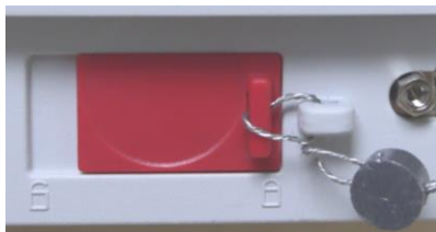
Locked with Wire Seal
